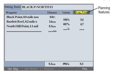
Press left or right on the ROCKER to select one of nine available planning features, including ETA (Estimated Time of Arrival at point), Fuel (to point), Leg Dist, Leg Fuel, Leg Time, Sunrise, Sunset (at point location), and Time To (point).
